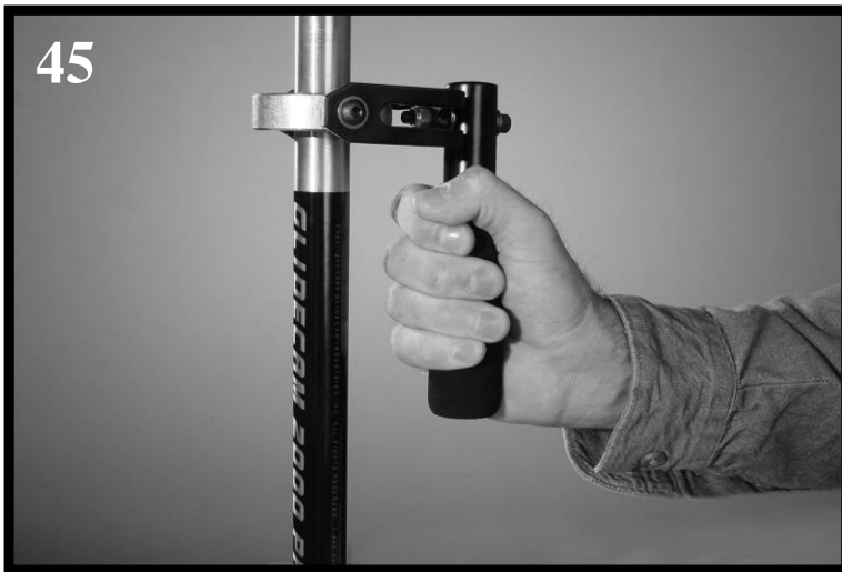
Photo #45 shows you the correct way to hold the handle; however, remember that you should always use both hands when using the HD-2000 as shown in Photo #46.
